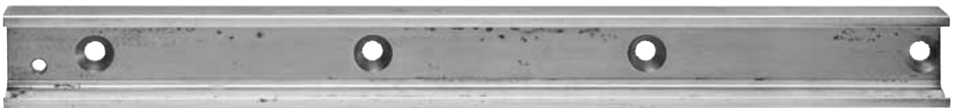
Coating Rollon Alloy after 720 hours
