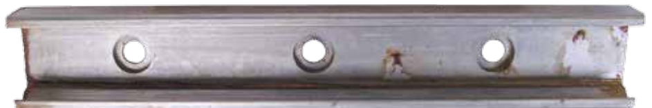
Chemical nickel plating after 360 hours
